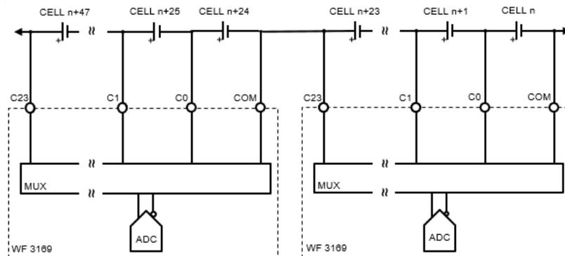
Figure 2. Using multiple WF 3169
