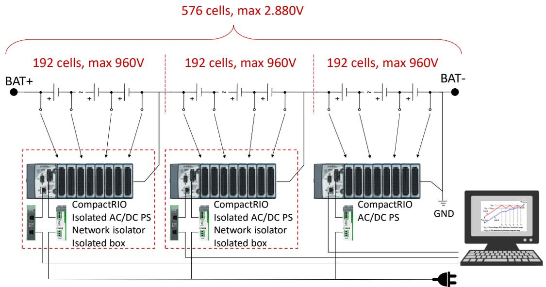
Figure 4. Setup with isolated CompactRIO chassis to enable measurements above 1000 volts
