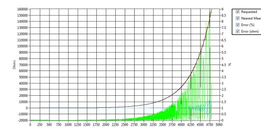
Figure 1. 5000 values distributed between 16  $\Omega$  - 160 k  $\Omega$  in Normal mode.
