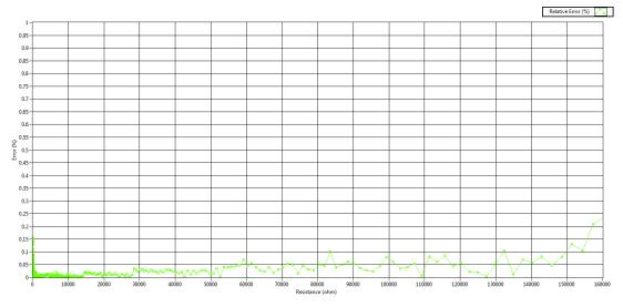
Figure 3. Error vs. Resistance in Enhanced mode.
