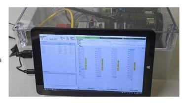
ignition pulse as well as the reference pulse using different slider bars in the GUI. It is also possible to manually change the RPM value while maintaining the pulse characteristics, i.e. the position and duration regardless if it is given in time- or CAD-domain.
