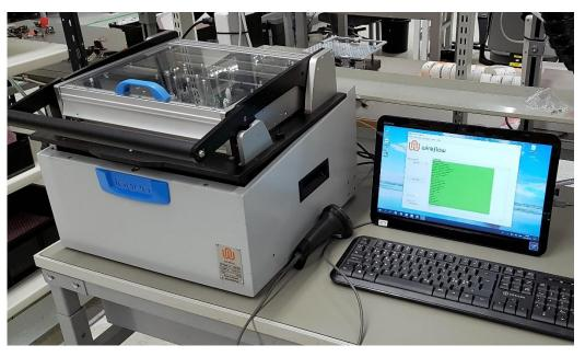
*Figure 4: Complete production tester setup with fixture to the left, hand scanner in the middle and the controller PC to the right.*
