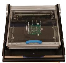
*Figure 2: Test object mounted in the cassette*
