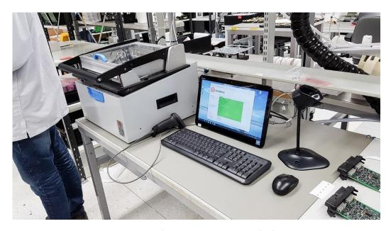
Figure 1 Test- and programming station in the factory
