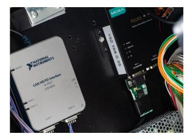
Figure 6 An I/O-box containing CAN and isolated RS232 interfaces
