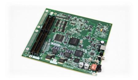
Figure 1 The USB-6001 OEM Multifunction I/O Device from National Instruments
