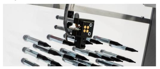
Figure 5 A light probe mounted on the pressure frame unit next to the pushrods
