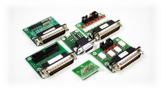
Figure 3 Signal conditioning boards, including three solid-state relay boards
