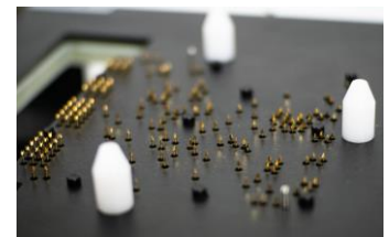
The plate is lowered which makes the needles come up and connect to the board
