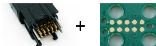
Figure 9 Solution for accessing test points with a connector interface fixture
