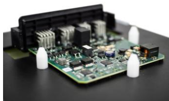
The board is placed in correct position on the plate by the board guides
