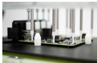
The pressure frame is closed and the pushrods are fixing the board
