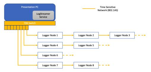
Figure 4. The logger network can be a mix of star- and daisy-chain topologies
