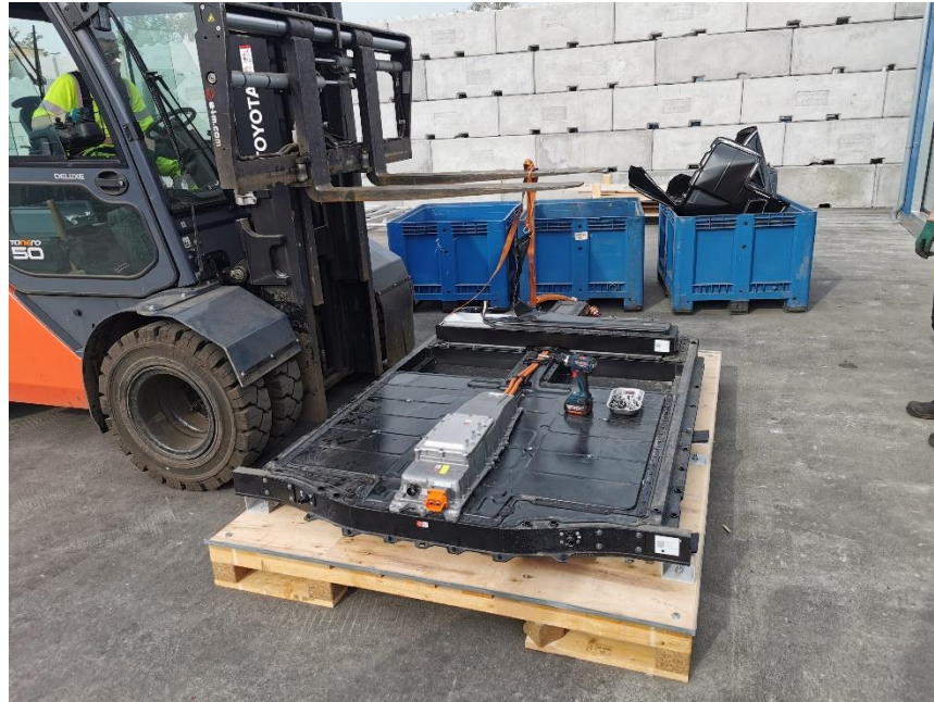
Figure 2 - A Porsche Taycan battery pack ready to be disassembled.
