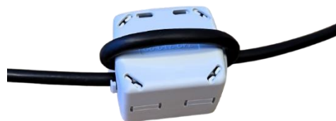
Figure 14 EtherCAT cable goes two turns in the ferrite
